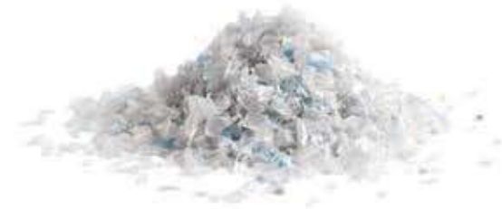
1 Plastic bottles are shredded into flakes.
