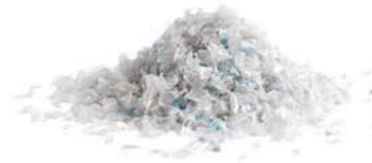
1 Plastic bottles are shredded into flakes.
