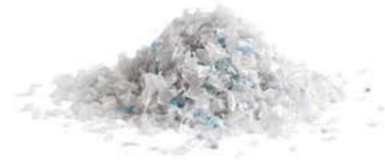
1 Plastic bottles are shredded into flakes.
